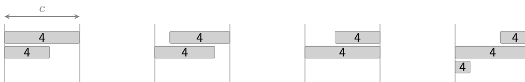
■ Figure 4 Modular representation of a long task assigned to a parallel workstation (task 4 from Figure 3), illustrating how it 'curls around' the cycle boundary. In each sub-figure the task is scheduled one more time-unit to the right.
